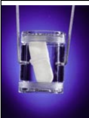
Wakame capsule after 2 hours in stomach acid and 1 hour in intestinal fluid
