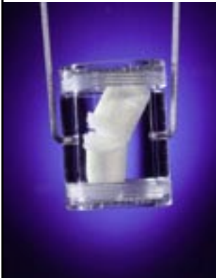
Wakame capsule after 2 hours in stomach acid and 2 hours in intestinal fluid
